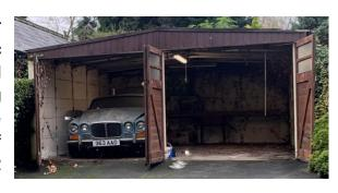
The car was all intact apart from the battery, the washer bottle and bracket had all been removed. I looked under the vehicle, which was inside a dry garage, with all the tyres original Dunlop radial tyres which had seen better days, all under inflated
